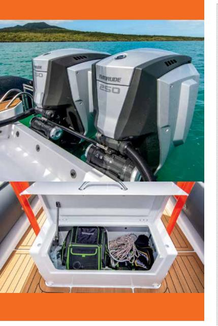
Stepping over the transom gets you to the massive boarding platform, and despite a pair of 250hp outboards there is still plenty of space to walk or stand between the engine cowlings and the transom. This is helped by the very neat cabling serving the engines the single cowled tube exiting from the sides does not impinge on the transom walkway.
