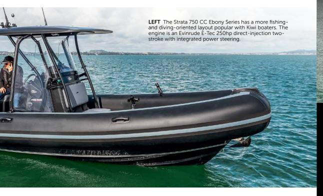
work of any chop, cushioning and coddling their occupants. Any tenderness at rest you might expect from such deep vee hulls is eliminated by the inflatable pontoons, which contact the water's surface when the boats are stationary, plus a 150-litre flooding chamber along the keel, which empties as the boat gets underway. Moulded hull strakes quickly lift the pontoons clear of the water to reduce drag and tabs combat any inclination to lie over to one side.
