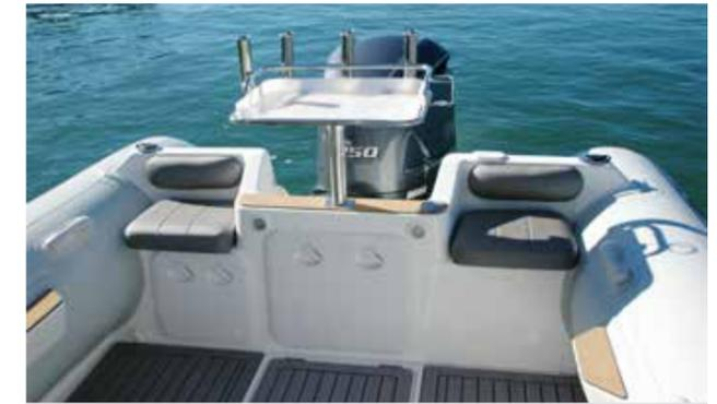
There's a live bait tank to port and battery to starboard.
