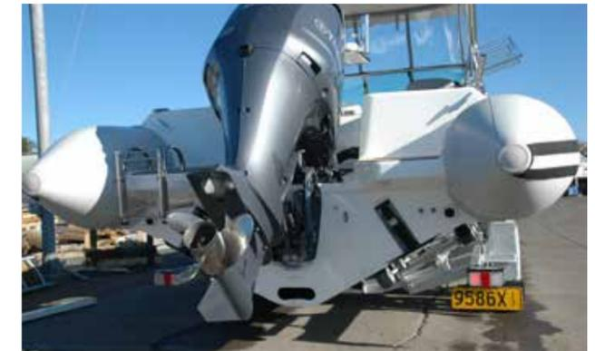
The 780 SuperSport is based on a 27 deg V hull with water ballast.
