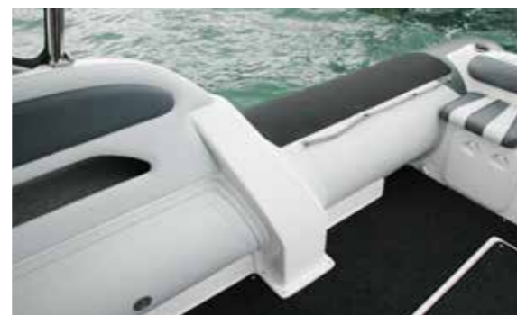
Deck supports secure the deck to the hull. Note the deep toe kicks and hard wearing surface on the tubes.
