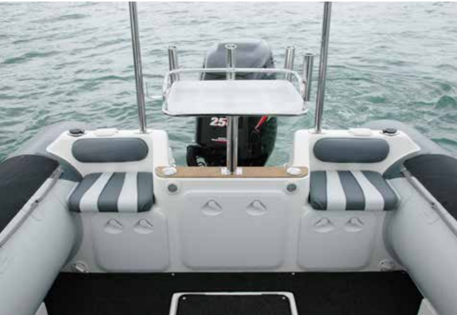
Above: Storage lockers under the aft deck also keep the twin batteries tucked away. Note the scuppers either side.
